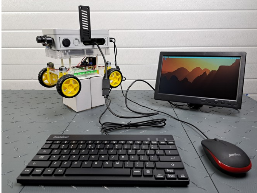
Figure 27 – Suspend R22 robot to prevent movement while testing motor control and direction
